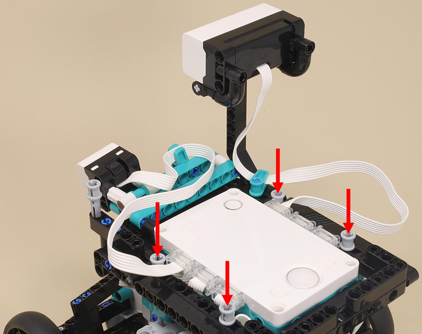
The arm wire should remain loose so the arm can unfold.
