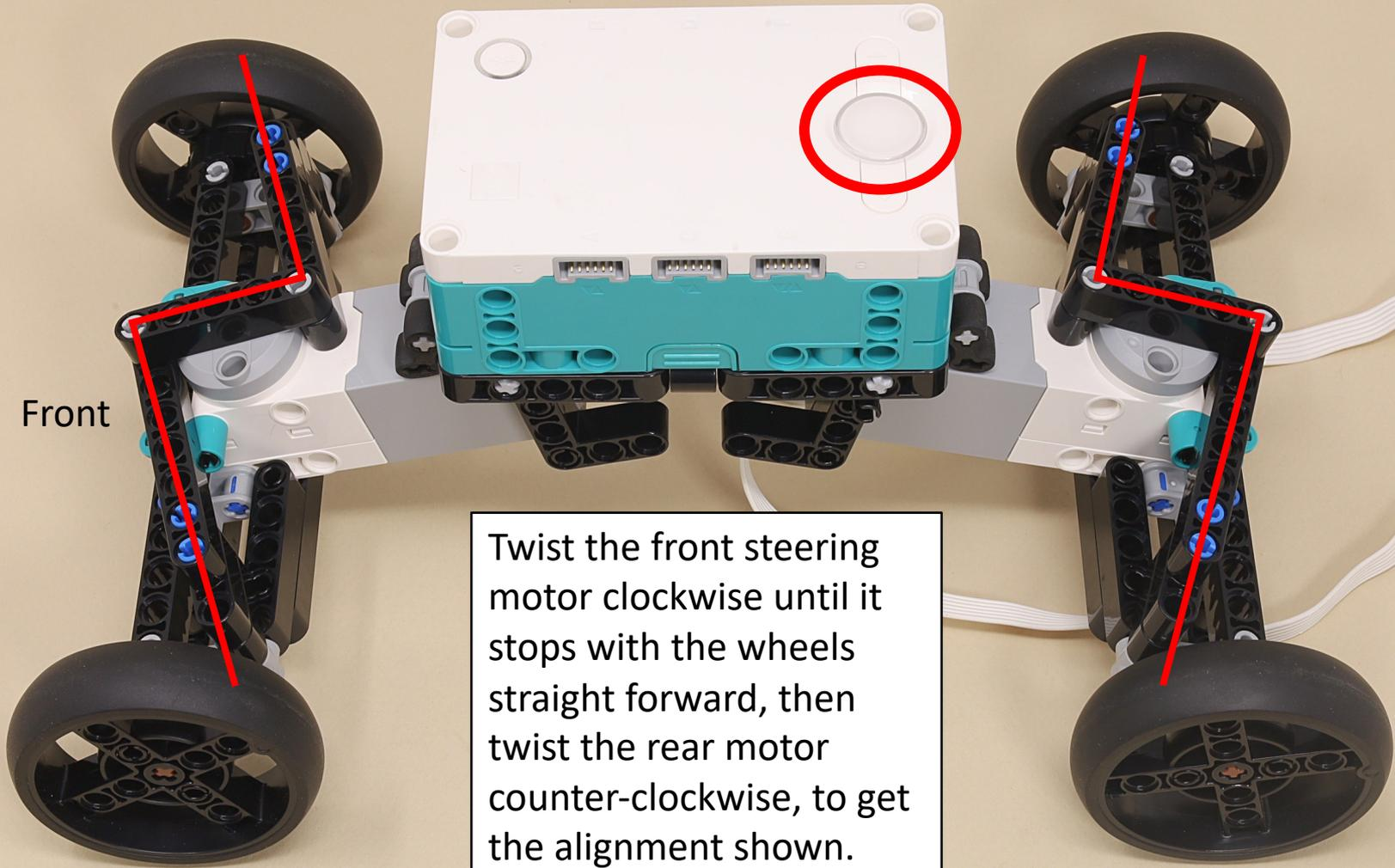
Twist the front steering motor clockwise until it stops with the wheels straight forward, then twist the rear motor counter-clockwise, to get the alignment shown.
