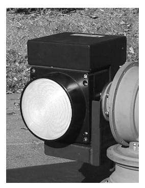
**Figure 6.** Close up of IDS radar on the MDARS-E turret.
