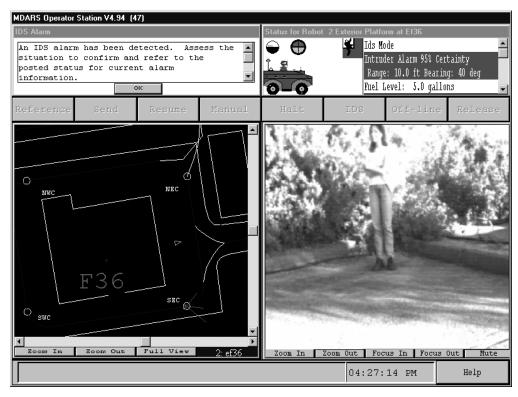
Figure 5. MRHA Operator Station Display depicting an IDS Alarm for exterior robot #2.
