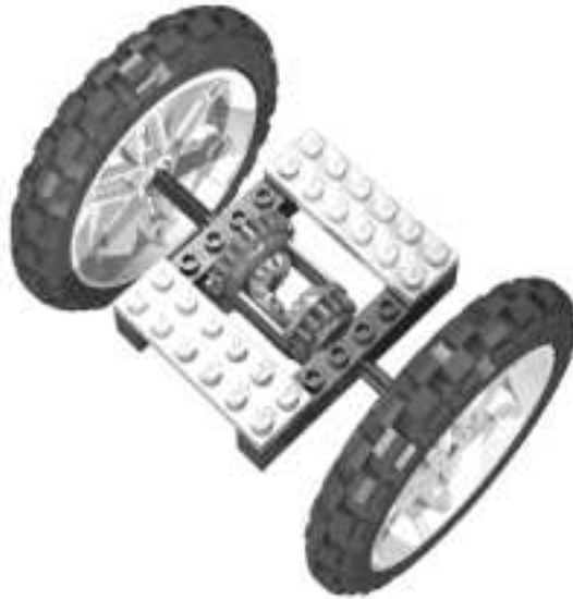
Figure 2.22 Connecting Wheels with the Differential Gear
