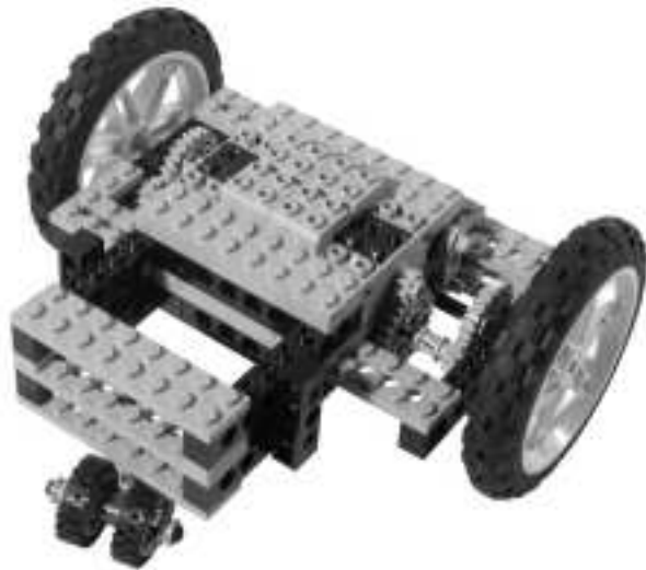
Figure 24.6 The Differential Drive that Controls Motion
