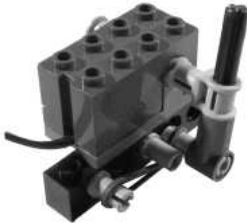
Figure 4.10 Emulating a Touch Sensor with a Rotation Sensor
