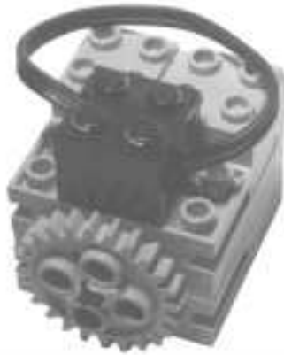
Figure 3.11 In This Setup, the Motor Shaft Turns Smoothly
