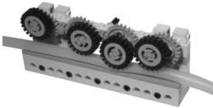
Figure 25.15 A Possible Setup for an Indirect Pumping Technique
