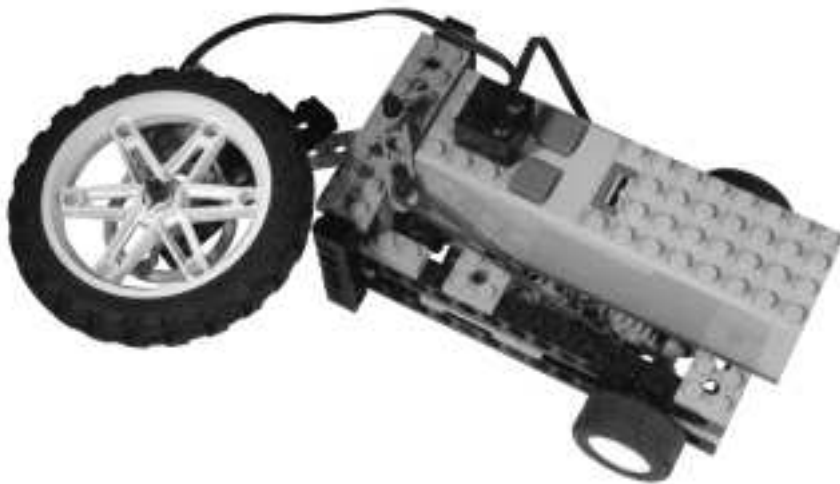
Figure 19.10 A Purely Mechanical Wall Follower
