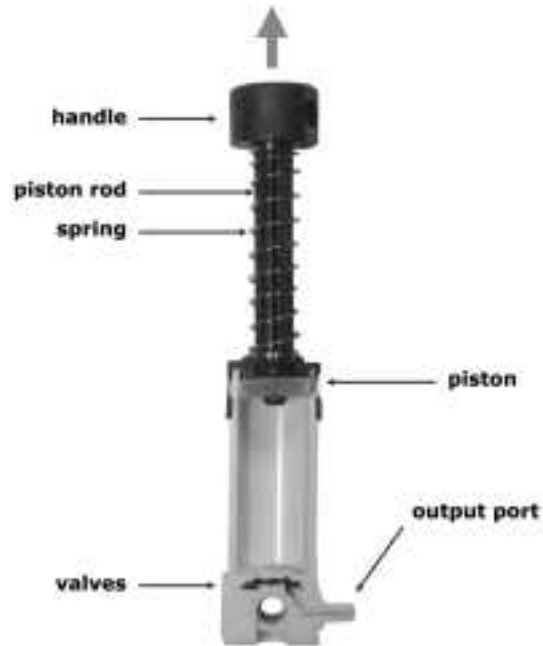
Figure 10.2 Cutaway of the Large Pump in Action
