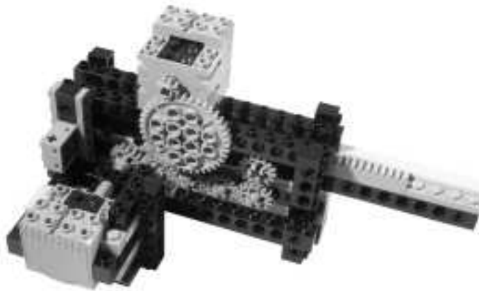
Figure 9.26 Switching a Motor among Five Output Axles
