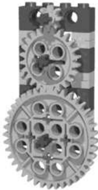
Figure 2.7 Vertical Matching of Gears
