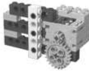
Figure 3.3 A Motor Connected to a Worm Gear
