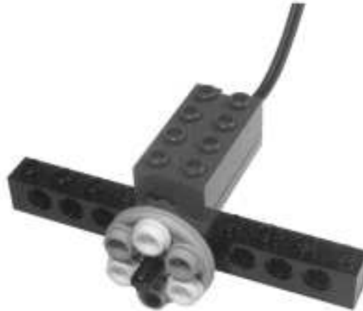
Figure 4.12 Emulating a Rotation Sensor with a Light Sensor
