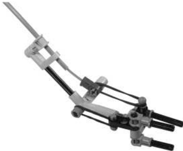
Figure 11.8 The Flex System Helps in Making Lightweight Hands
