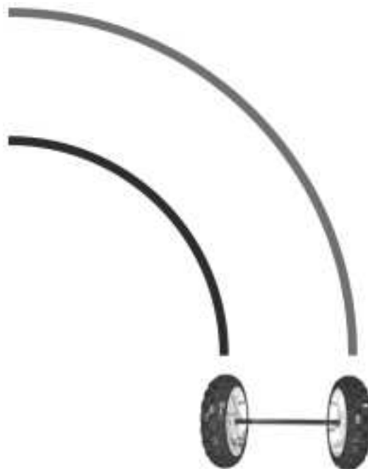
Figure 2.21 During Turns the Wheels Cover Different Distances
