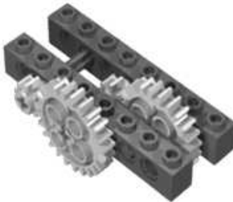
Figure 2.3 A Geartrain with a Resulting Ratio of 1:9
