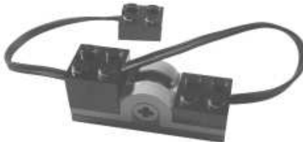
Figure 4.13 Emulating a Rotation Sensor with a Polarity Switch
