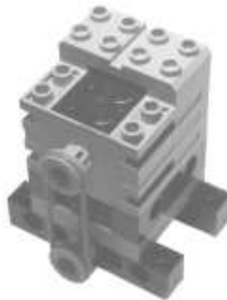
Figure 3.6 Belts Don't Require Very Solid Mountings
