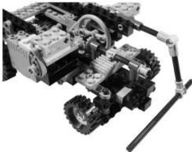
Figure 14.19 Detail of the Rack and Pinion Steering Assembly
