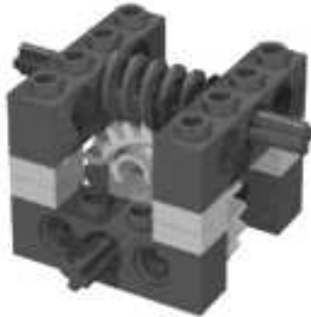
Figure 2.4 A Worm Gear Engaged with a 24t
