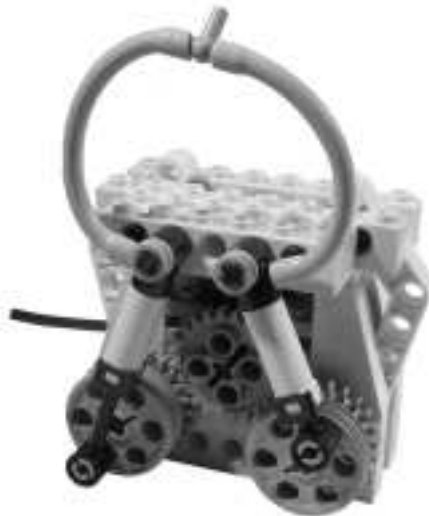
Figure 10.13 Ralph Hempel's Double Acting Compressor
