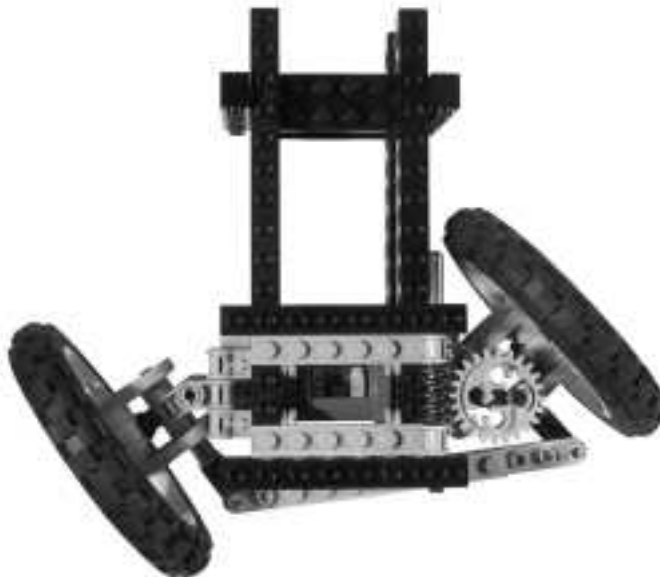
Figure 14.26 This Design Features Ackerman Correction
