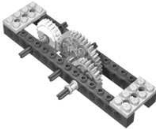
Figure 2.6 Placing the Clutch Gear in a Geartrain
