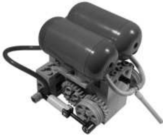
Figure 10.14 Another Double Acting Compressor
