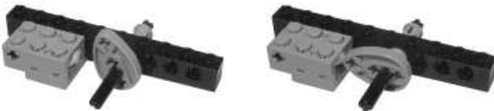
Figure 4.11 Emulating a Rotation Sensor with a Touch Sensor
