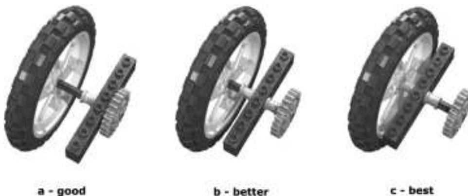
Figure 5.5 Keep a Wheel as Close as Possible to Its Supporting Beam
