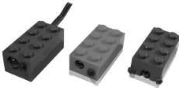
Figure 9.12 Different Kinds of Infrared Proximity Sensors
