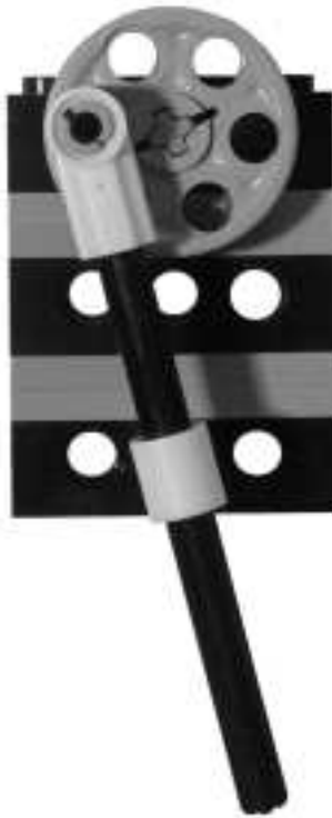
Figure 15.13 This Leg Describes an Ellipse
