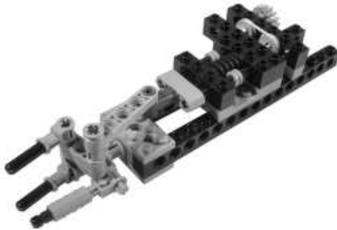
Figure 11.2 This Small Hand Uses Linear Motion
