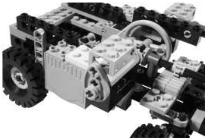
Figure 14.21 The Touch Sensor that Monitors the Steering
