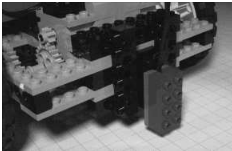
Figure 14.8 Set the Proper Distance between the Sensor and the Pad
