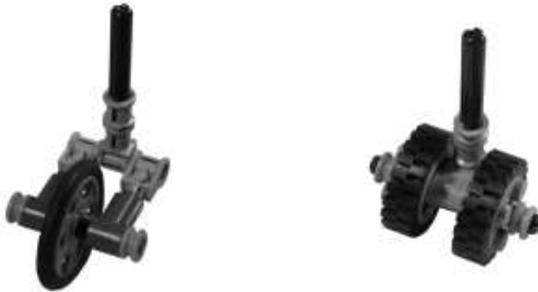
Figure 8.6 Casters Designed to Avoid Skidding
