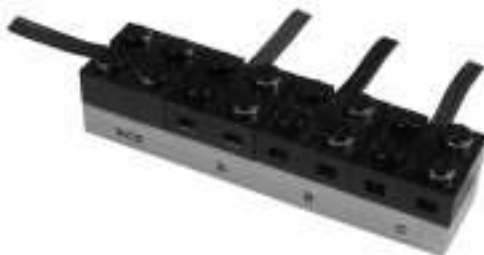
Figure 9.19 A Three Touch Sensor Multiplexer
