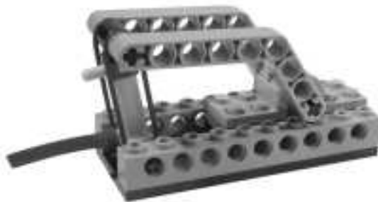
Figure 10.15 A Pressure Switch
