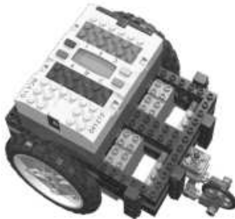
Figure 5.11 Poor Positioning of the Load RCX Makes This Robot Unstable
