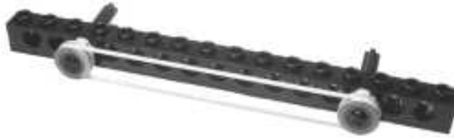
Figure 2.18 Pulleys Allow Transmission across Long Distances
