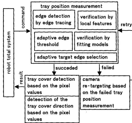
Figure 10. software configuration of tray position measurement and tray cover detection
