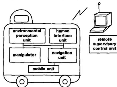
Figure 2. The components of the robot
