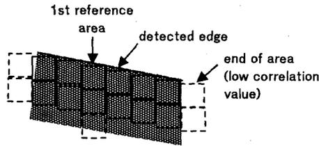
Figure 14. parallelogram area detection using adjacent correlation operation
