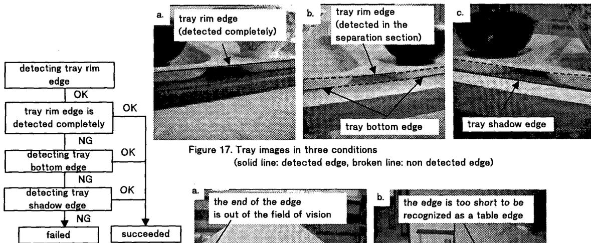
Figure 16. sequence of adaptive target edge selection
