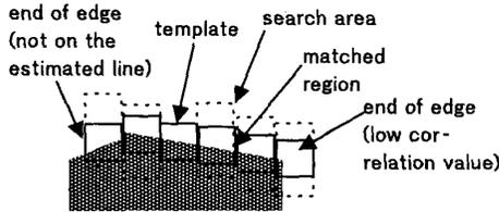
Figure 12. edge detection using adjacent correlation operation
