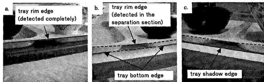
Figure 17. Tray images in three conditions (solid line: detected edge, broken line: non detected edge)
