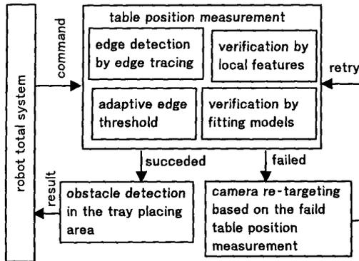
Figure 9. software configuration of table position measurement and obstacle detection
