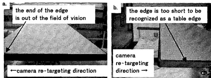
Figure 18. examples of failed camera targeting
