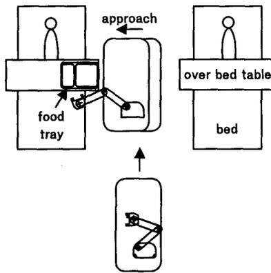
Figure 3. Movement of the robot at bedside
